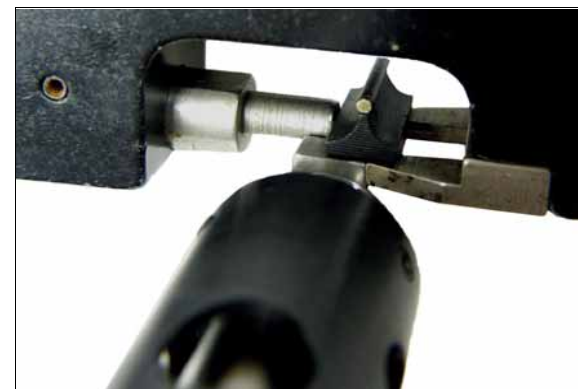
1. Drift out the factory front sight.
